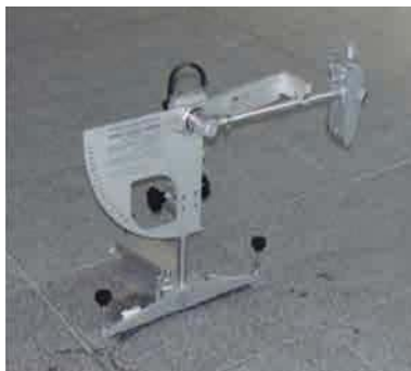
Pendulum Test Machine (image courtesy of HSE)
